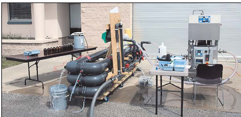
Photo 1. Pilot-Scale Ozone Unit
